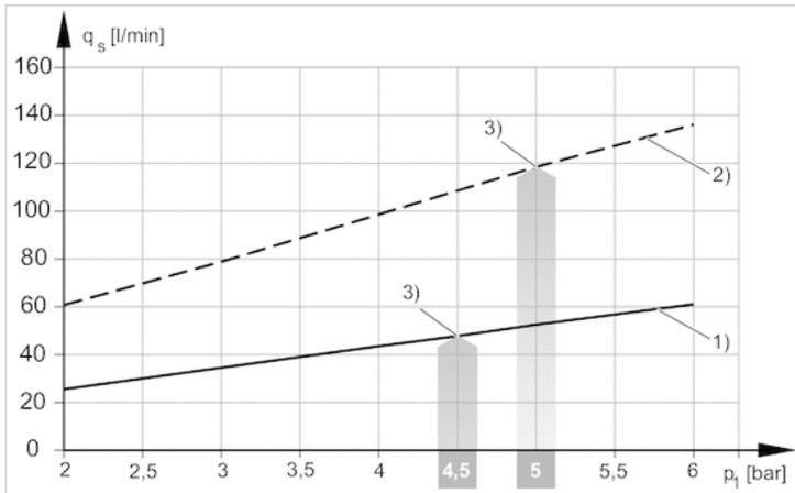
1) = Ø Düse 1,0 mm 2) = Ø Düse 1,5 mm
