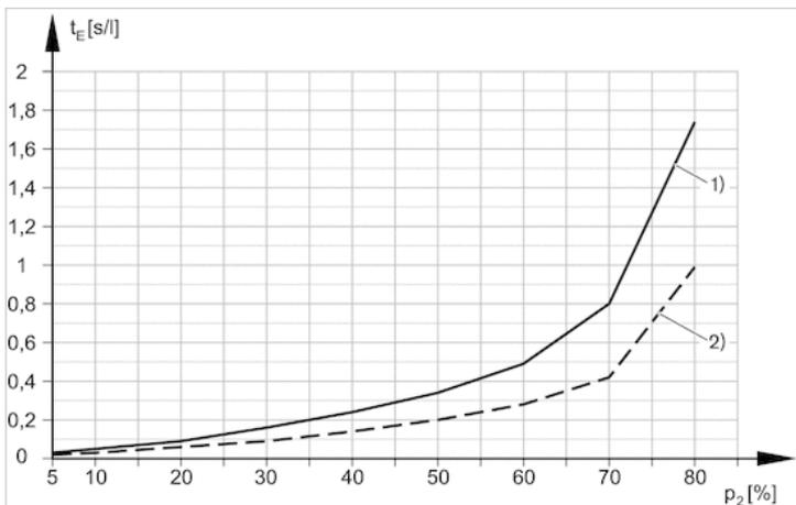
1) = Ø Düse 2,0 mm 2) = Ø Düse 2,5 mm
