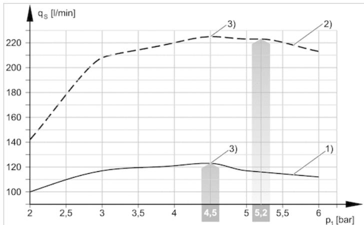
1) = Ø Düse 2,0 mm 2) = Ø Düse 2,5 mm
